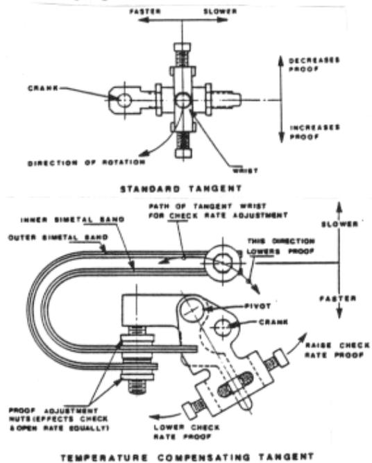
**Figure 3. Tangent Adjustments**
