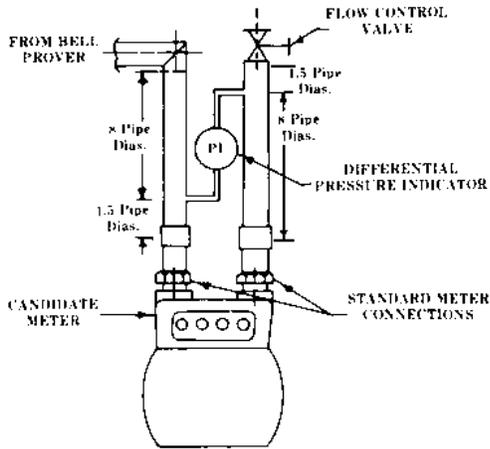
**Figure 4. Test Apparatus**
