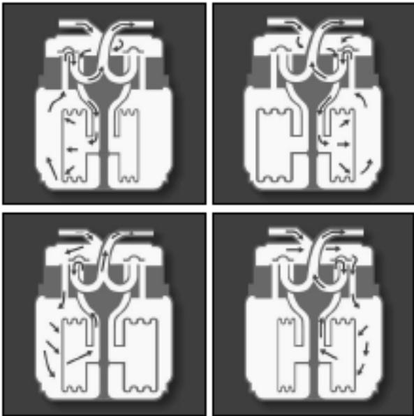
**Figure 1. Glover Four-chamber Diaphragm Meter Flow Paths.**
