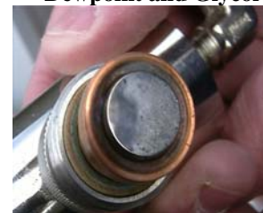
Mirror outside of Instrument coated With Glycol
