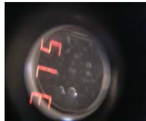
Large amount of Hydrocarbon Liquids on Mirror
