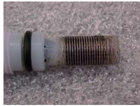
P 2 O 5 contaminated With Glycol
