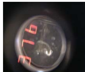
Glycol & Liquid Hydrocarbons On Mirror
