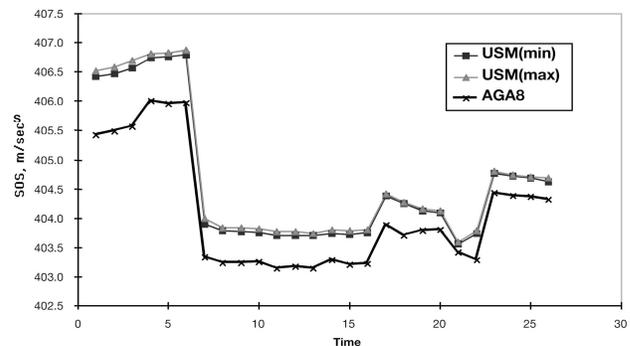
FIGURE 2. 8-INCH METER MEASURED VS. CALCULATED SOS
