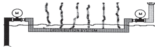
FIGURE 1. Leakage in a gas system can have an effect on unaccounted-for gas.
