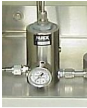
Figure 1; Pneumatic Injection Pump
