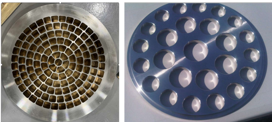
Figure 6: Photo of Less Restrictive Flow Conditioner vs. More Restrictive Original Flow Conditioner
