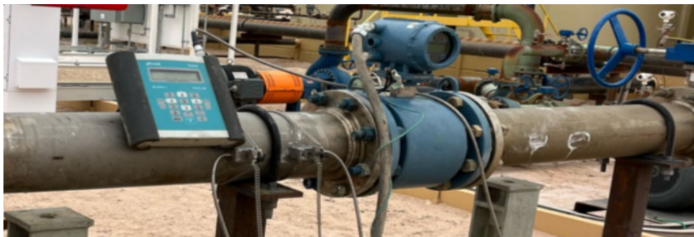
Figure 5. Clamp-on ultrasonic validation of a produced water meter
