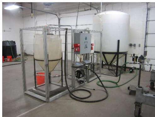
Figure 5: ISO 17025 certified gravimetric water draw test stand – Flow MD – Phoenix, AZ
