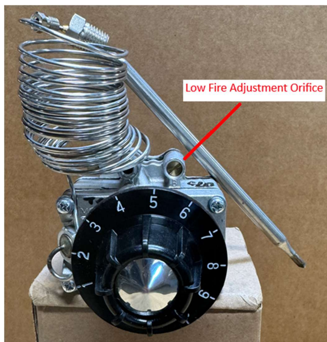
Figure 14: Example temperature controller showing the location of the low fire adjustment orifice
