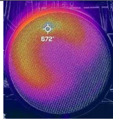
Figure 4: Gas valve opened after 15 minutes. Notice warmer spot where gas is catalyzing
