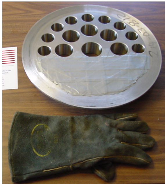
Figure 4 – 40% Blocked Flow Conditioner
