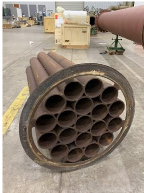
Figure 11 19-tube bundle flow conditioner
