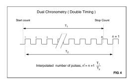
Timer 1 is stopped when the final detector switch is actuated (This is the time for displacing the known
