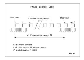
A frequency Rf is generated which is a fixed constant R above the flowmeter frequency. The pulses of Rf are counted between the actuation of the first detector and the final detector. The totalized pulses are then divided by R to obtain the interpolated pulses.
