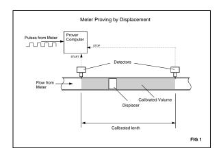
When sizing meter provers one of the main criteria is that counting meter pulses during the proof run must not contribute more than 0.01% to the overall uncertainty of the proving results. This requires a minimum resolution of 1 part on 10,000.
