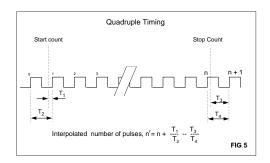
Times  $T_1$ ,  $T_2$ ,  $T_3$ , and  $T_4$  are derived from the same high frequency oscillator.
