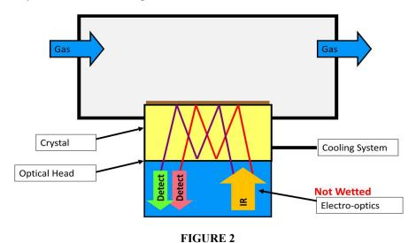
CEIRS<sup>TM</sup> not only accurately and unambiguously detects the onset of condensation, but it also can characterize the nature of the condensate. This is due to the fact that absorption is monitored at different wavelengths. Thus, one can distinguish between a hydrocarbon dewpoint and a water dewpoint. This is an added advantage of this technique.
