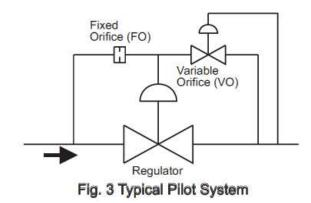
Another important element in a discussion of Pilot systems is Proportional Band. Proportional Band is the inverse of GAIN and can be defined as the percent drop in set pressure as a regulator goes through its full range of operation, or
