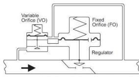
Fig. 5 Loading Type Pilot Operated Regulator
