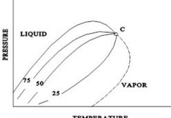
TEMPERATURE FIGURE 3: PHASE DIAGRAM OF A MIXTURE
