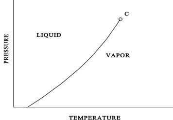
FIGURE 1: PHASE DIAGRAM OF A PURE SUBSTANCE
