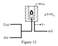
The second direct method utilizes principles of the residual oxygen measurement. This is a flameless technology that measures the excess oxygen from a continuous stream of sample gas which is oxidized in a catalytic converter. The sample gas and air mixture from the fuels conditioning system is catalytically combusted in an oven whose temperature is set to approximately 812°C and by a thermocouple and PID algorithm programmed in the microcontroller. Figure 13.
