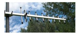
FIGURE 6. Typical Yagi Antenna
