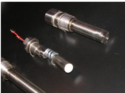
Figure 6 Transducer Assembly and Housing
