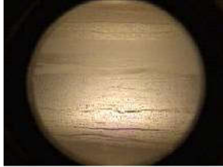
Fig 26. CEESI wet gas view port of wet gas flow upstream of DP Flow meter.
