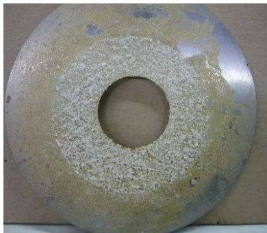
Fig 21. A heavily contaminated DP Flow plate.
