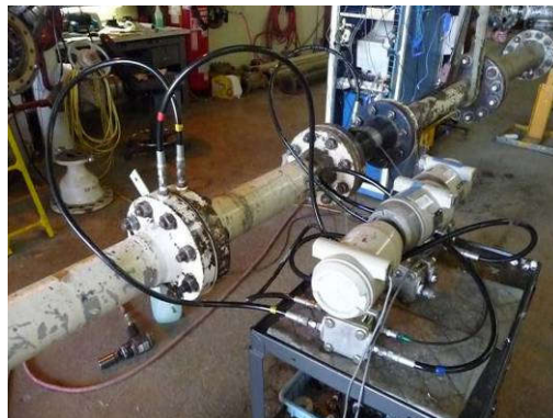
Fig 5. Flange installed plate with air flow.
