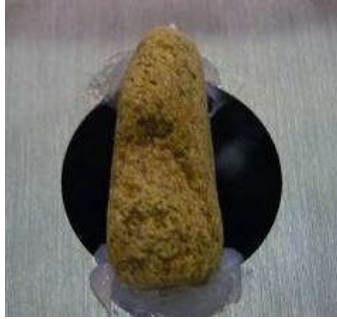
Fig 29. Rock trapped at an DP Flow plate.
