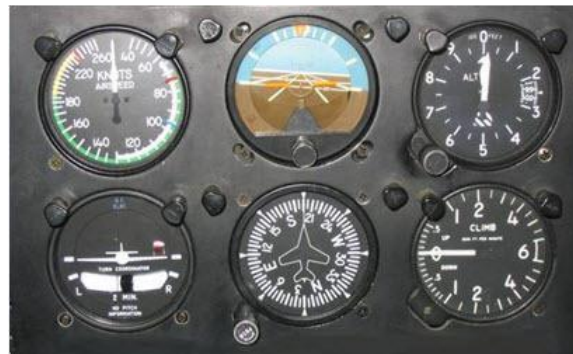
Figure 3. Sacred Six Instruments in Cockpit
