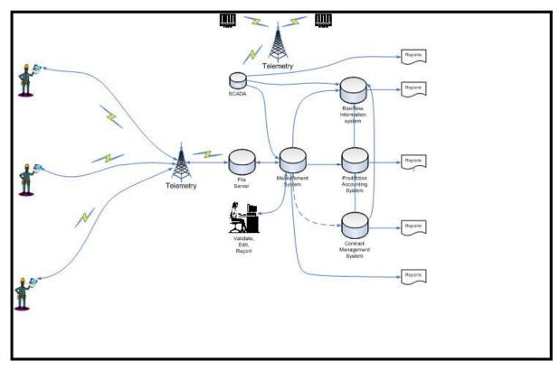
Figure 4. Automated Field Data Capture - Data Flow
