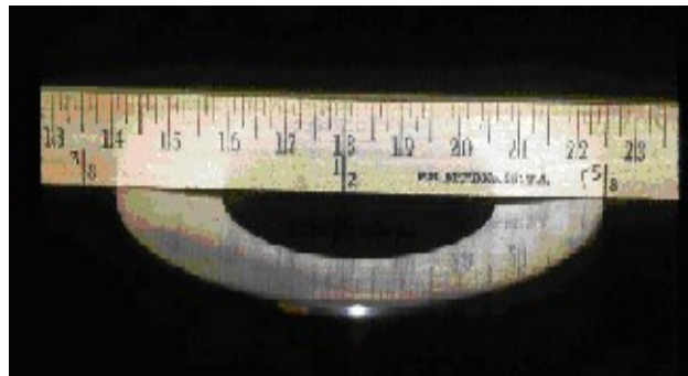
FIGURE 3. Orifice Plate Buckled by a Slug Strike
