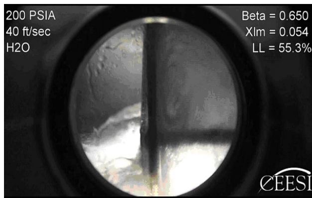
FIGURE 4. Stratified Flow Through an Orifice Plate
