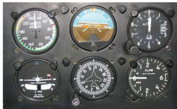
Figure 3. Sacred Six Instruments in Cockpit
