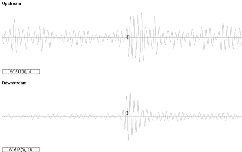
**Figure 4. Ultrasonic Noise from a Regulator Downstream of the Meter**
