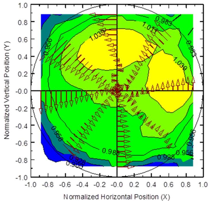
**Figure 2. Contours of Measured Velocity Values 10D Downstream of Two Out-of-Plane Elbows**
