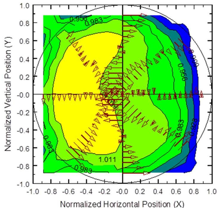
**Figure 1. Contours of Measured Velocity Values 10ND Downstream of a Single Elbow**
