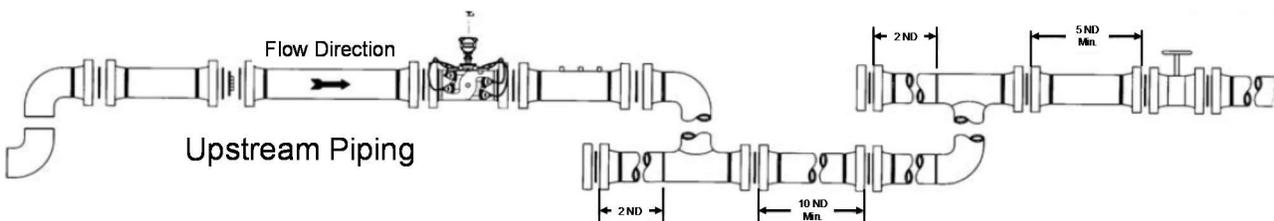
**Figure 5. Piping Geometry to Reduce Ultrasonic Noise Transmission**
