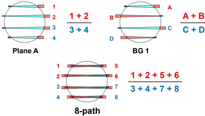
Figure 19 Asymmetry Calculations for different path designs
