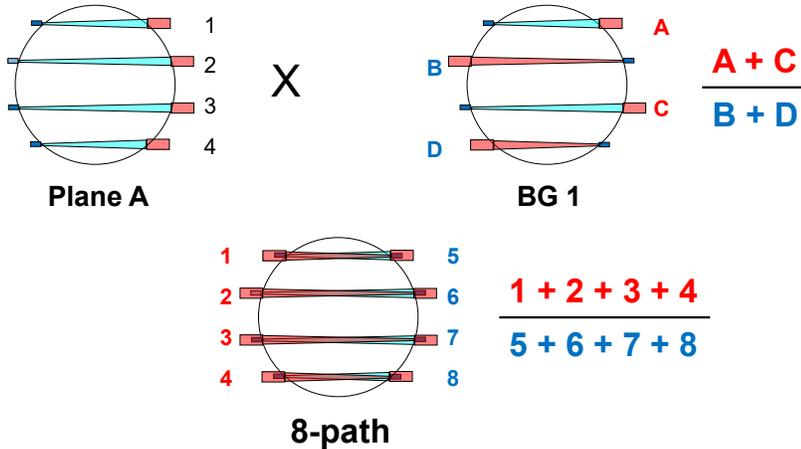
Figure 20 Plane Balance or Cross Flow Based upon different path designs
