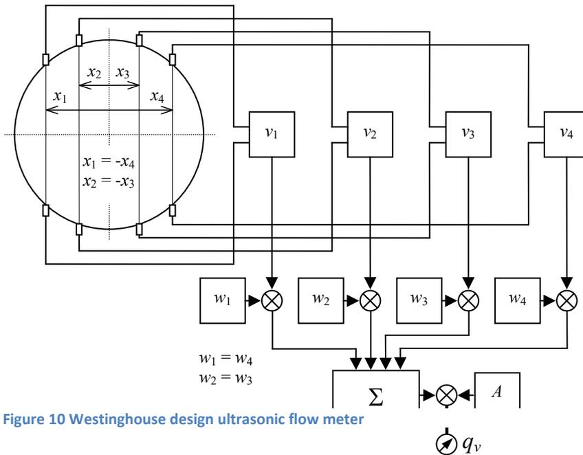
Figure 10 Westinghouse design ultrasonic flow meter
