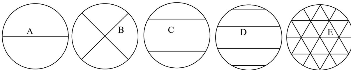
**Figure 7 Possible transducer arrangements for Spool piece meters**
