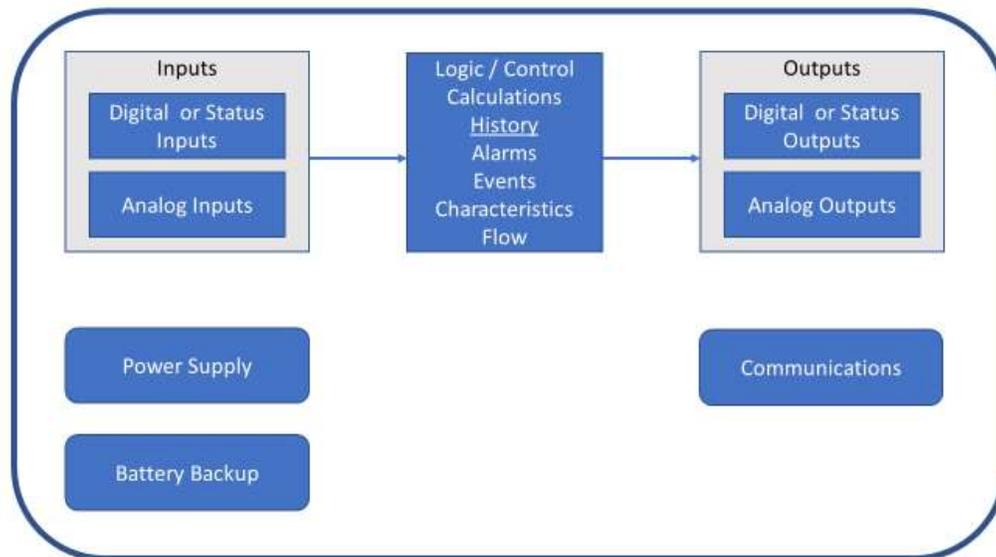
**Figure 2. Example Electronic Flow Computer System Architecture**
