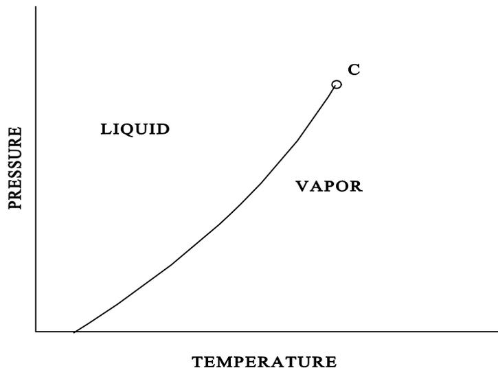
FIGURE 1: PHASE DIAGRAM OF A PURE SUBSTANCE
