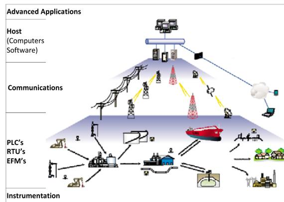
**FIGURE 1. Five Logical Levels of a SCADA System**
