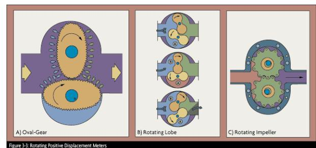
Figure 8 – Schematic of Typical Positive Displaced Meters
