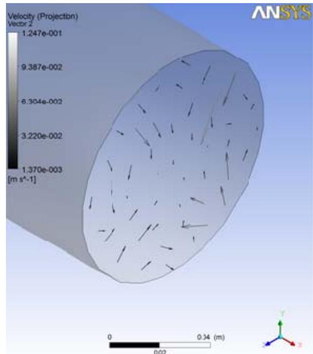
Figure 4 – Product Swirl from Installation Effect with Flow Conditioning
