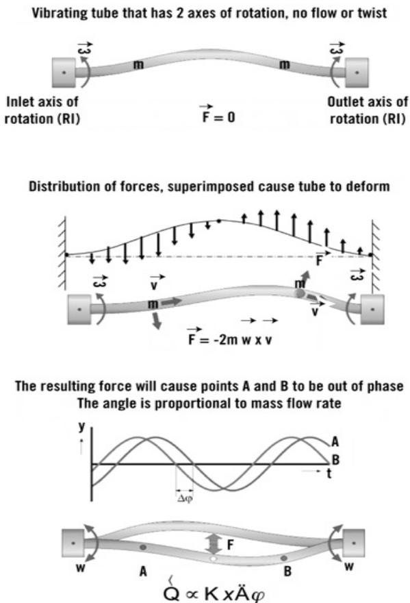
Figure 9 – Schematic of Coriolis Meter Guiding Principles
