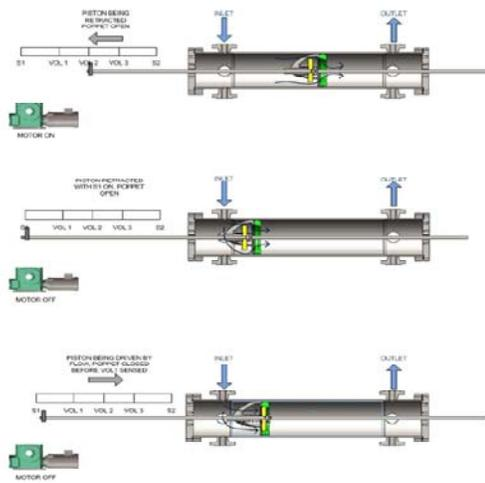
Figure 11 – Typical Prover Operation
