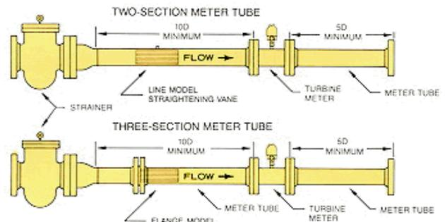
Figure 5 – Meter Tube with Strainer and Flow Conditioning
