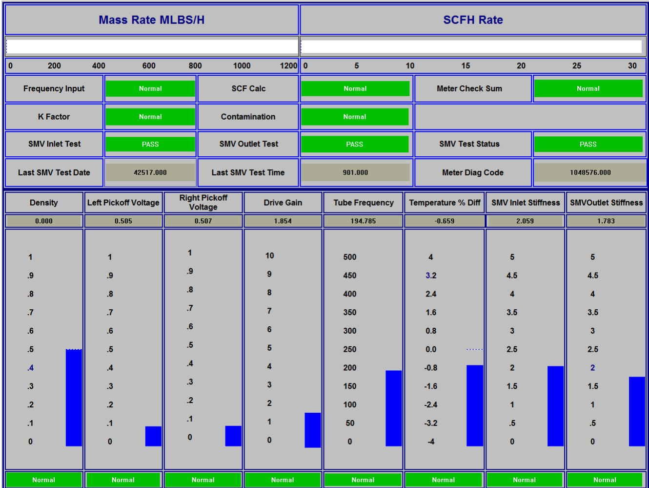
Figure 14, ADMS Field Device Coriolis Overview.
