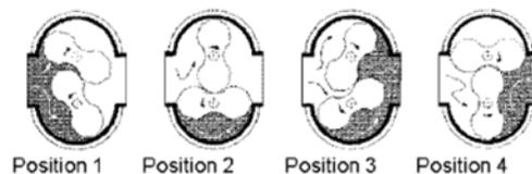
**Figure 1. ROOTS Rotary Positive Displacement Operating Principle**
