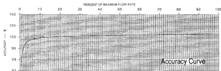
**Figure 2: Typical Accuracy Curve**
