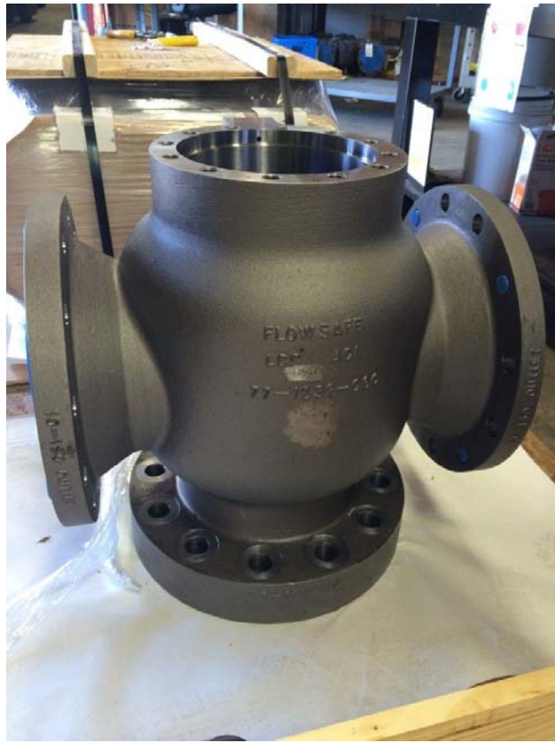
Figure 9. PRV Body during Scheduled Teardown Inspection
