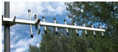
**FIGURE 5. Typical Yagi Antenna**
