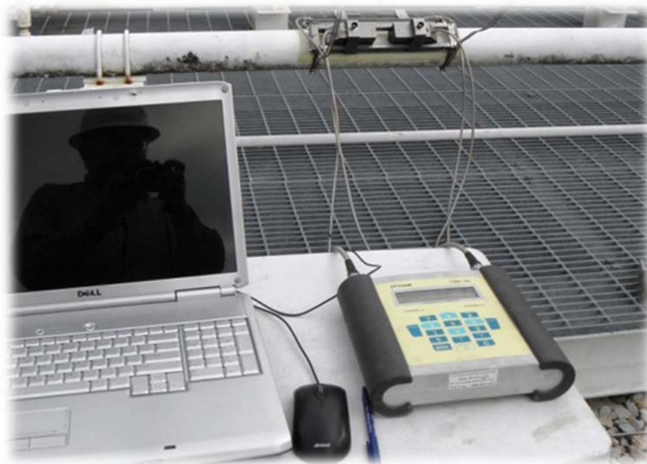
**Figure 4 - CLAMP-ON METER INSTALLED ON PIPE**
