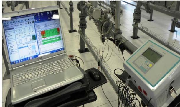
**Figure 10 - Siemens Clamp-On and Sick USM**
