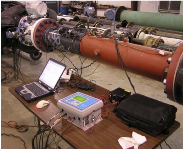
**Figure 15 - CLAMP-ON REFERENCE AT CUSTODY METER CALIBRATION**
