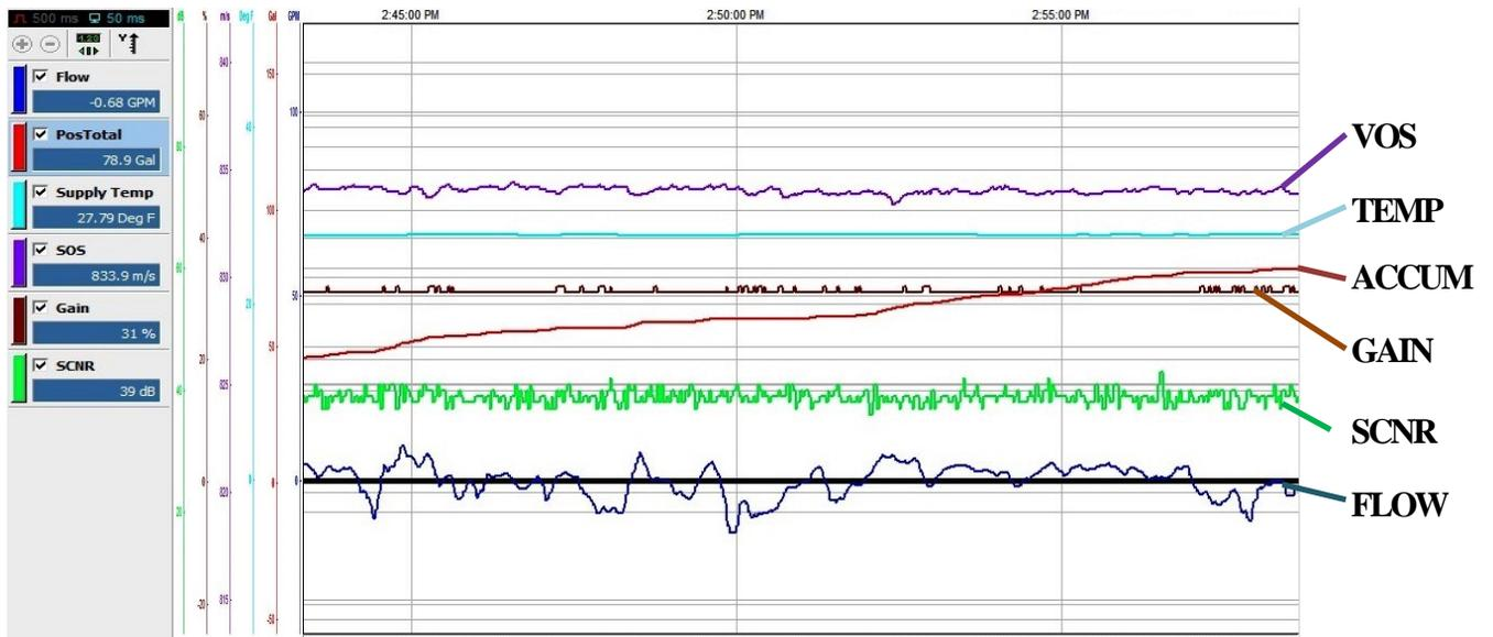
**Figure 3. - REAL TIME DATA FROM CLAMP-ON METER**
