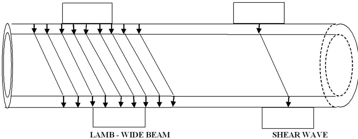
**Figure 1 - TRANSDUCER TYPES**
