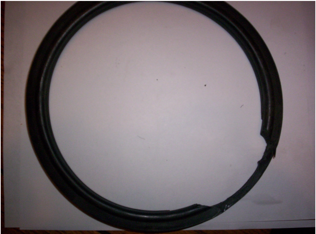
FIGURE 5. Torn Seal Ring
