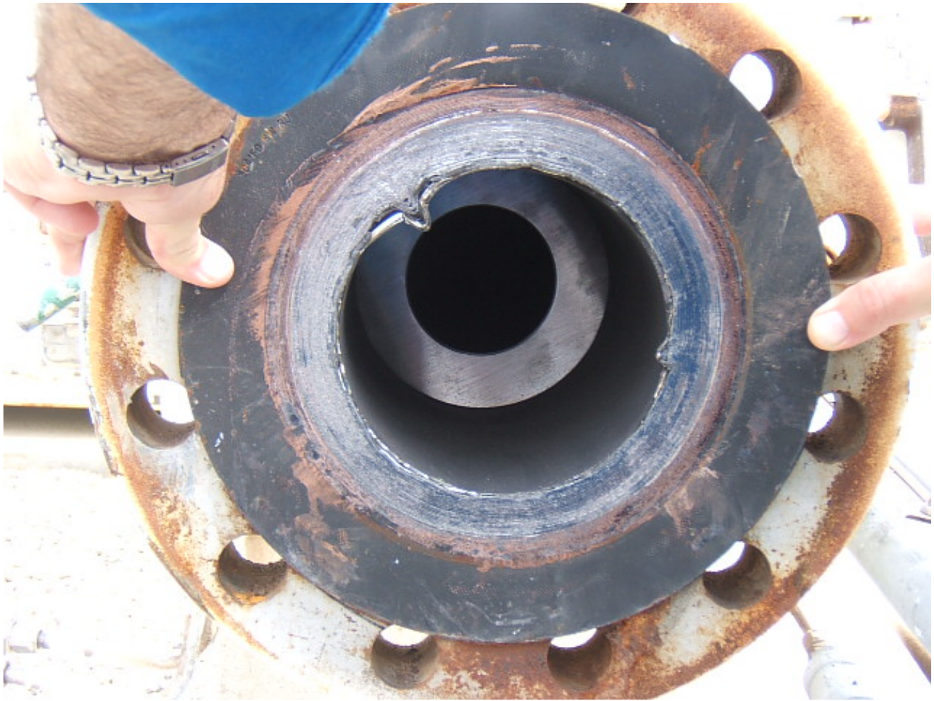
FIGURE 6. Incorrect Gasket Size Example
