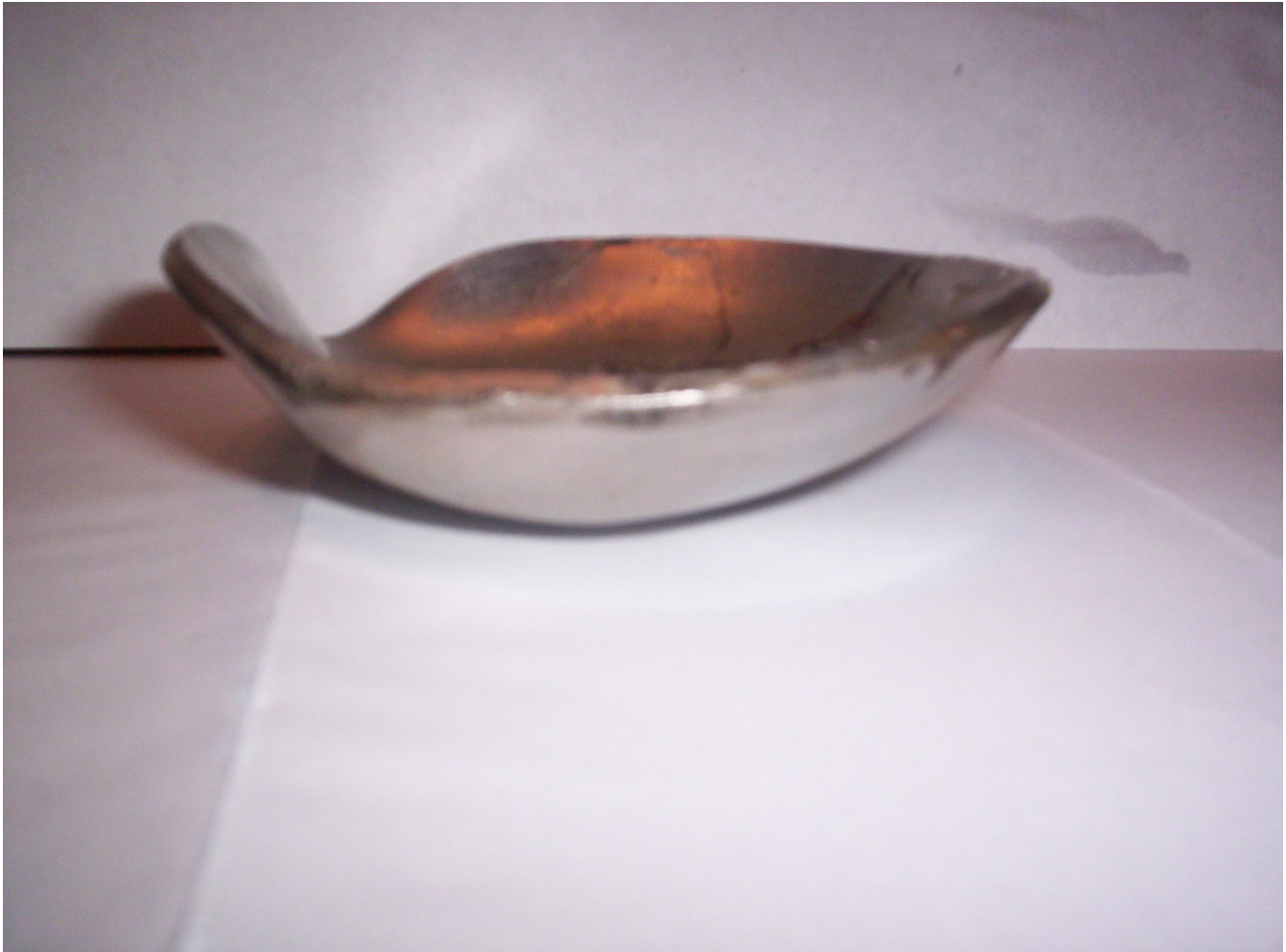
FIGURE 4. Orifice Plate Damaged by Loose Straightening Vanes
