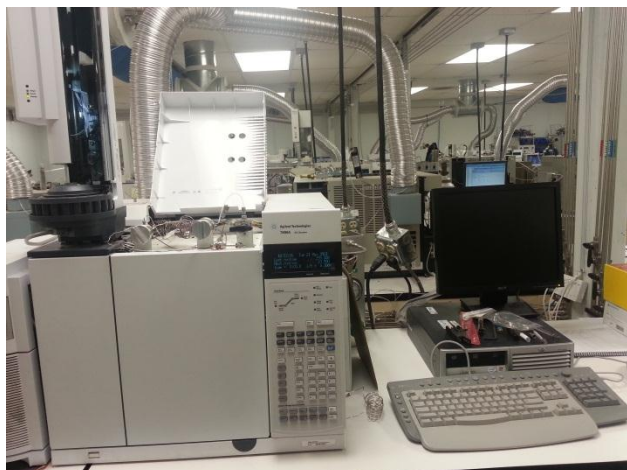
Figure 3. Gas Chromatograph set up for the certification process
