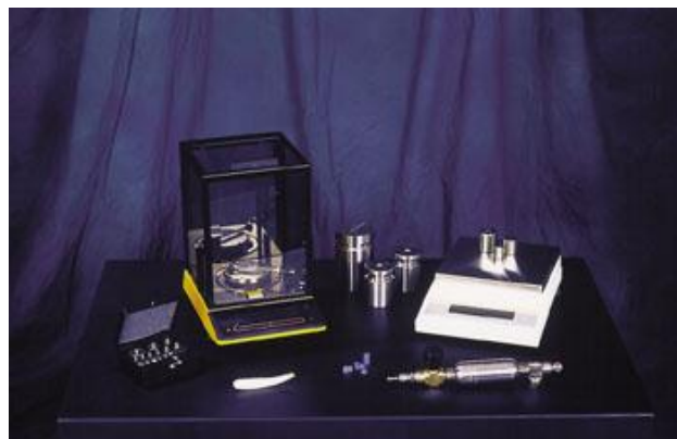
Figure 2. Balances and masses used to gravimetrically prepare calibration standards
