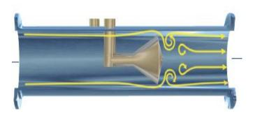
The centrally located cone inside the meter body reshapes the profile of the flow as it enters the meter body. The cone can have many different diameters which makes most "Cone Meters" a fixed Beta Ratio. The principle of the meter is similar to that of the Orifice Meter and the Venturi Meter, using a Beta Ratio. As the flow comes into contact with the cone, it creates a low pressure region just downstream of the cone. See illustrations below:
