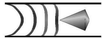
This pressure difference can incorporate the Bernoulli equation to determine a flow rate. This unique design and how it changes the profile of the gas as it enters the meter without a flow conditioner assures accurate and repeatable measurement even with harsh upstream conditions. Little or no upstream piping required.
