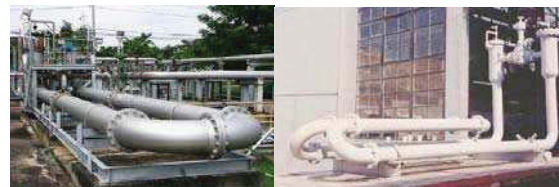
Figure 7: Examples of Pipe/Ball Provers
