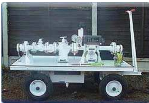
Figure 6: Master Meter Test Cart
