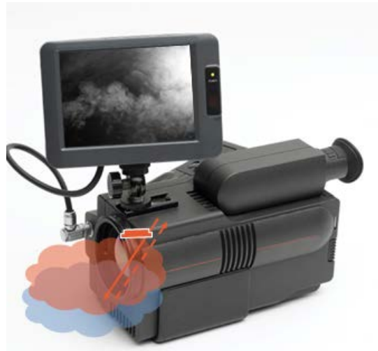
Figure 5: Video Image of Gas Leak
