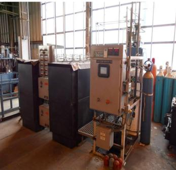
Figure 1. Cylinder bake out ovens used in the preparation of cylinders.
