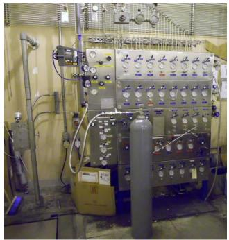
Figure 2. Blending panel used in the gravimetric preparation of calibration standards.
