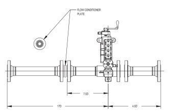
Figure 10. Required Upstream and Downstream Straight Pipe Lengths Specified in API MPMS Chapter 14.3 for a Perforated plate Type Flow Conditioner Installation.
