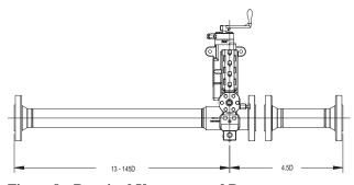
Figure 8. Required Upstream and Downstream Straight Pipe Lengths Specified in API MPMS Chapter 14.3.
