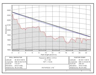
Above: A path study using professional software, confirms if a good path—exists and also indicates how to point the antenna correctly. This is the Azimuth.
