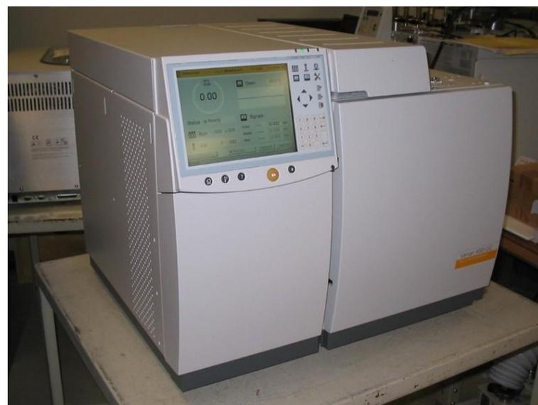
**Figure 3.** Typical gas chromatograph (GC) used for analytical certification of calibration standards.
