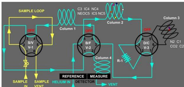
**Figure 3 - Valve 3 timing will separate C2 and smaller components from the C3 and larger components. When the retention times increase while the valve timing stays fixed, not all of the C2 may make it into Column 3 before the valve switches.**
