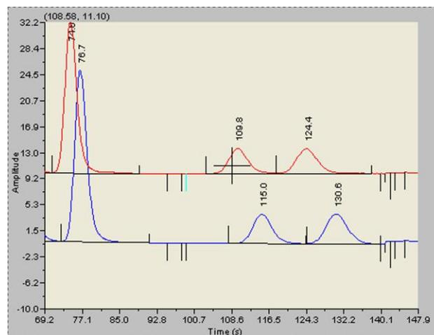
**Figure 4 - Retention time shift highlighting the potential for mis-measurement during the next period of operation. The latest chromatogram is shown in blue, and the chromatogram from the last verification test is shown in red.**
