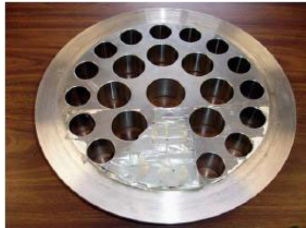
Figure 22 – 3 Holes Blocked Flow Conditioner
