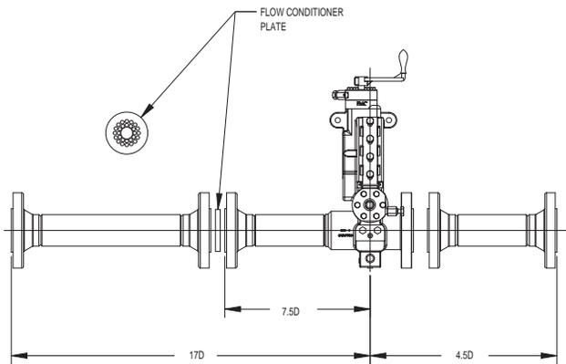
**Figure 10. Required Upstream and Downstream Straight Pipe Lengths Specified in API MPMS Chapter 14.3 for a Perforated plate Type Flow Conditioner Installation.**
