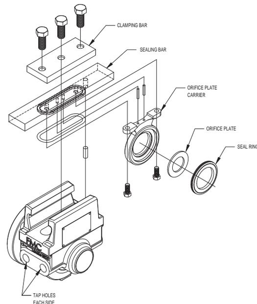
**Figure 4. Principal Components of a Single Chamber Orifice Fitting**
