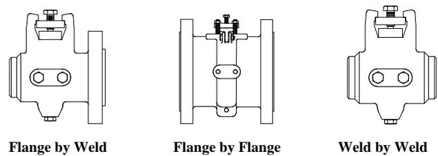
**Figure 3. Single Chamber Orifice Fitting Configurations**
