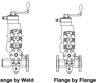
**Figure 6. Dual Chamber Orifice Fitting Configurations**
