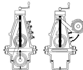
**Figure 7. Dual Chamber Orifice Fitting Configurations**
