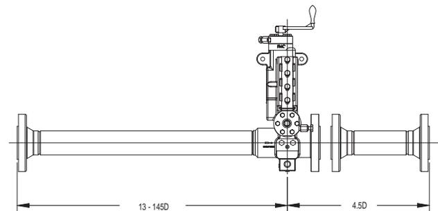
**Figure 8. Required Upstream and Downstream Straight Pipe Lengths Specified in API MPMS Chapter 14.3.**
