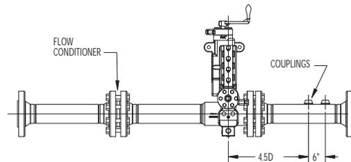
**Figure 11. Required Upstream and Downstream Straight Pipe Lengths Specified in API MPMS Chapter 14.3 for a Perforated plate Type Flow Conditioner Installation.**
