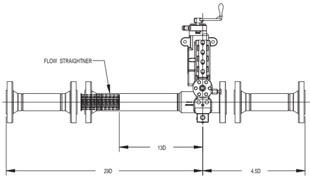
**Figure 9. Required Upstream and Downstream Straight Pipe Lengths Specified in API MPMS Chapter 14.3 for a 19-Tube Bundle Flow Conditioner Installation.**
