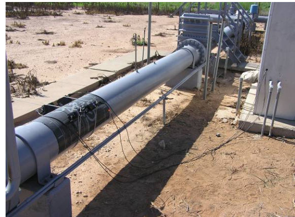
Figure I. Clamp-on Compared to Orifice Meter
