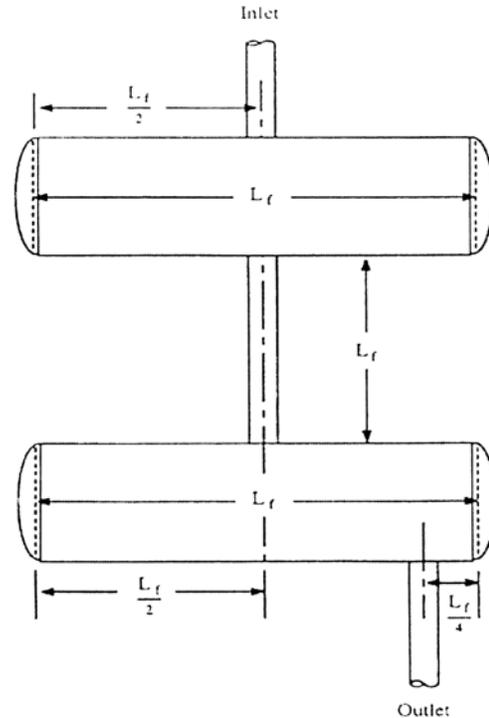
FIGURE 1. TWO BOTTLE LOW-PASS ACOUSTIC FILTER
